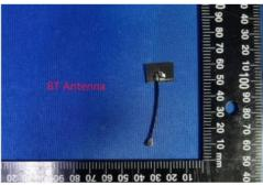
2.4G WIFI (2400-2500MHz) antenna gain is 0.52dBi and 0.48dBi.
