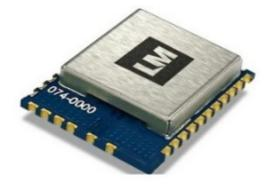
The WC5EM2601F is a complete dual-band(2.4GHz and 5GHz)WIFI 2×2 MIMO module. This module provides a high level of integration with a dual-stream IEEE 802.11n MAC/ baseband /radio. The WLAN operation supports 20MHz,40MHz, and 80MHz channels for data rates up to 300Mbps. It fully complies with IEEE 802.11 a/b/g/n/ac feature-rich wireless connectivity at high standards and delivers reliable, cost-effective, throughput from an extended distance.
