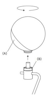
2. Insert the light bulb then gently mount the diffuser screwing it back to the metal ring.
