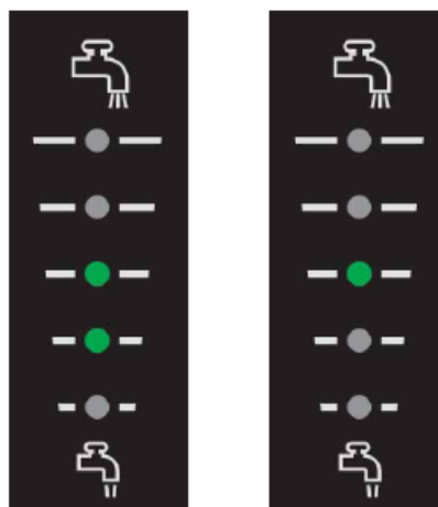
Fig. 14 SCALA2 outlet pressure indication
