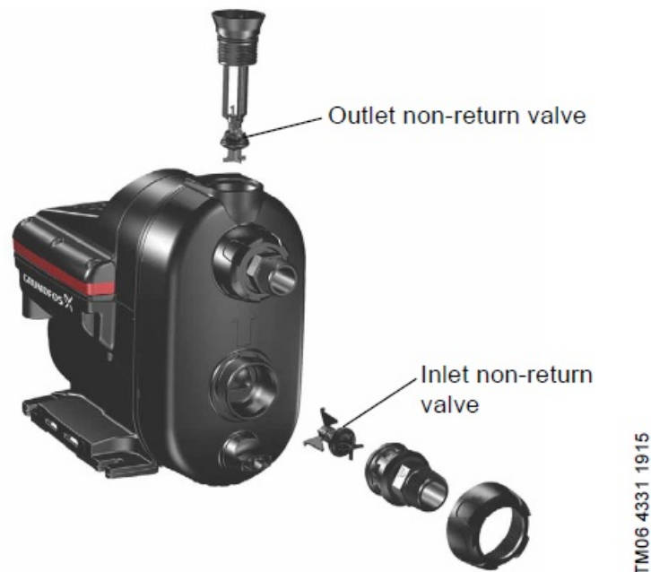
Fig. 20 Outlet and inlet non-return valves
