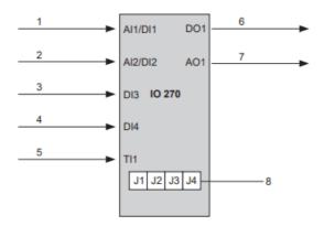
IO 270 I/O signals. Jumpers are used to configure analog input signal types and selection between AI1/DI1 and AI2/DI2. The digital inputs (DI1-DI4) are normally open (NO) contacts.
