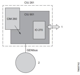
CIM 260 and IO 270 built into a CIU 261 and connected to a Grundfos product via GENIbus
