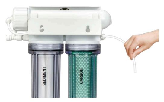
• Point this tubing down into a bucket or drain, and slowly turn on the incoming water supply. Carbon dust will start pouring out. Flush KDF carbon filters for at least 10 gallons.
