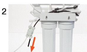
If you do not have a flush valve, then flushing can be done by disconnecting the drain line either before the ASV or at the flow restrictor. Make sure the feed water is turned OFF and the system is depressurized before attempting to remove the drain line connection. Follow the steps below.
