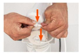
2. Install the new sediment and carbon filter, making sure they go into the correct filter housings.
