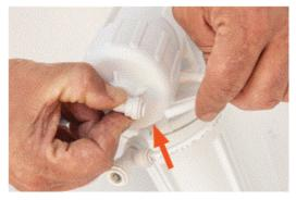
3. Pull out the membrane using needle nose pliers or another similar tool.
