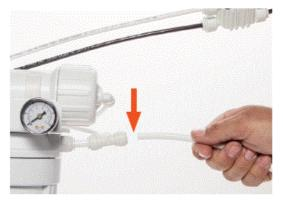
2. Connect the 1/4" white RO tubing to the auto shut-off valve, making sure the RO tubing seats into the quick-connect fitting. This is the filtered RO water outline.
