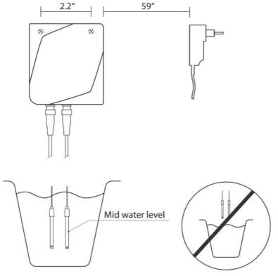
**Important notice:** Probes should NOT hang above the water level and must be submerged at all times. **C.** Installation is complete. Start growing!
