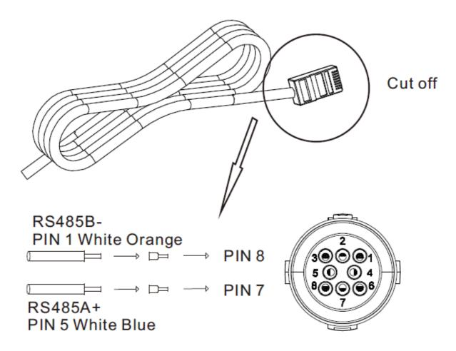
The standard RS485 cable length is 15m. If need longer RS485 cable, please use an ethernet coupler to extend and make sure RS485 cable less than 100m (the recommended length is less than 25m).
