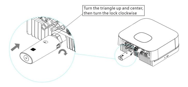
After the installation , if the LED light of Shine RF Stick-X flash quickly, it means installation works. If the LED light is off, please recheck the connection between Shine RF Stick-X and inverter.
