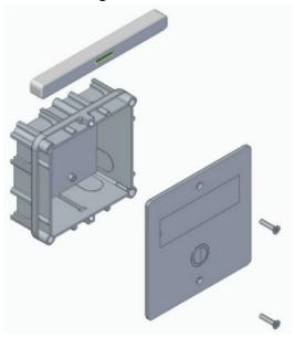
Insert the flush-mounted box into a mortar bed in the masonry using a spirit level and fix the storey plate to the flush-mounted box with the screws supplied.
