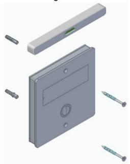
Align the surface-mounted adapter with the masonry using a spirit level and fasten it with the fastening material supplied.
