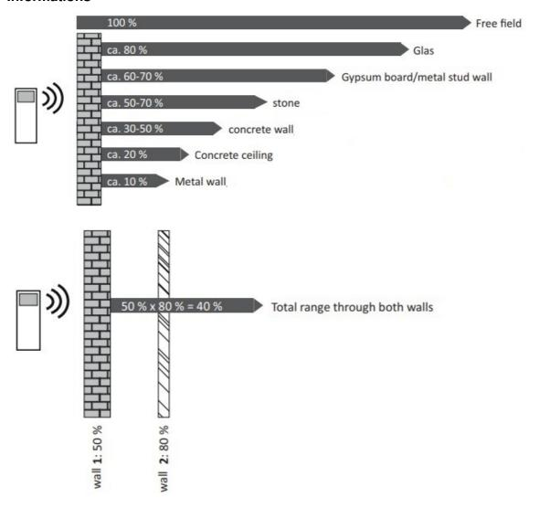
The range of the ETA Funk is approx. 250 m if unobstructed and if the transmitter is installed in accordance with the instructions. Walls, doors, metal components etc. may reduce the range significantly. See illustration below **Note:** the range can be significantly reduced with flush mounting, depending on the nature of the wall e.g. reinforced concrete.
