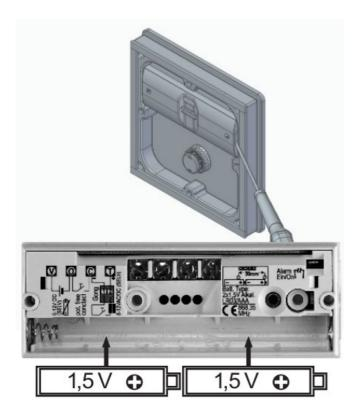
To open the transmier housing, place a sloed screwdriver in the grove on the transmier housing one aer the other on the right and le and turn it by 90°.
