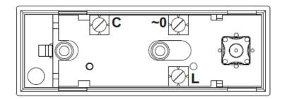
• Loosen the screw with a screwdriver. Insert the stripped wire under the plate and tighten the screw again.
