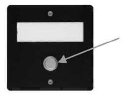
Put the MISTRAL, ECHO or CALIMA receiver into pairing mode. Please refer to the instruction for the relevant recipient. Operate the bu on on the ETA radio. The ETA is paired with the receiver.
