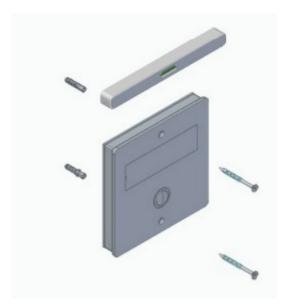
**Flush moun ng variant:** Insert the flush-mounted box into a mortar bed in the masonry using a spirit level and fix the storey plate to the flush-mounted box with the screws supplied.
