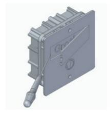
Open the Plexiglas cover with a screwdriver, insert the name tag inlay into the recess provided and carefully insert the Plexiglas cover.
