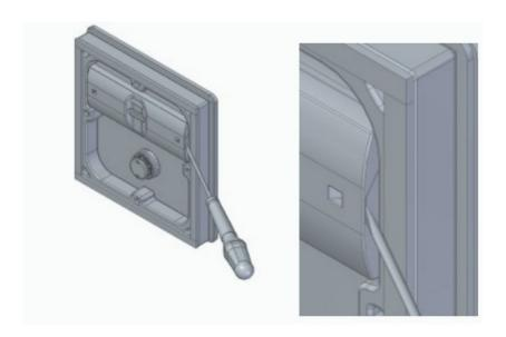
To open the transmit er housing, place a slo ed screwdriver in the grove on the transmit er housing one and the other on the right and le and turn it by  $90^{\circ}$ .
