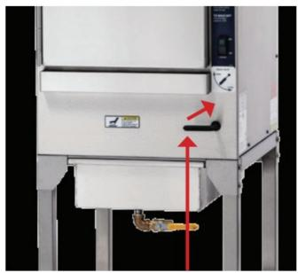
2. Once the reservoir has completely drained (approximately 5 minutes), stand to the hinged side of the door (Figure 2), slowly open the door allowing all of the steam to escape from the cavity. Allow the cavity to completely cool down and confirm that the reservoir has completely emptied before cleaning the overflow drain.
