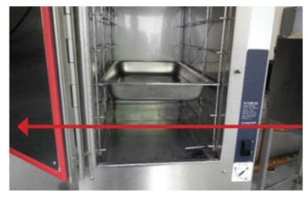
3. Remove the steam lid (Figure 3) and fan cover assembly (Figure 4), prior to cleaning the overflow drain.
