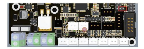
To use an external BIGTREETECH DCDC5V V1.0 module, short the pins shown in the above image using a jumper.
