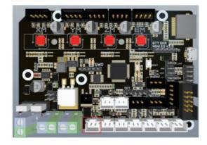
Connect the fan by FAN2 to realize the whole machine cooling. Please note that the operating voltage is the same as the input power supply voltage to avoid damage.
