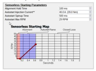
When a brushless motor is run without Hall sensors and started from a complete stop, the motor controller attempts to ramp up the motor's rpm to a minimum speed so that it can latch onto the rotation (closed loop). It does this by first injecting a static current into the phase windings to orient the motor into a known position. The controller then rotates this field faster and faster until reaching the "Autostart Max RPM" value.
