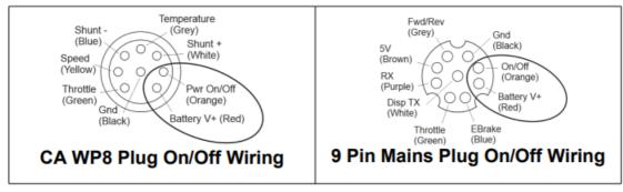
In order to power on, the Phaserunner V6's on/off wire must be shorted to battery V+, through either the WP8 plug or the 9 pin mains plug. This is accomplished either with a Cycle Analyst plugged into the WP8 plug, or one of the 9 pin mains cable options on the 9 pin plug. If battery power is applied without the on/off input connected to V+, the controller won't turn on or connect to a computer.
