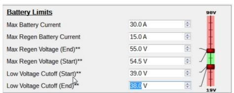
With the controller mapped to your motor and spinning correctly, you should now set the battery voltage and current settings to appropriate values for your pack.
