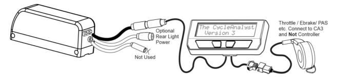
The 6 pin PAS plug of the controller is typically not used in this arrangement except as a possible Fwd/Rev input source. The 9 pin Mains cable either can be left unterminated, or it can be used as a power tap for running rear lights, using a 9 to 2 pin power adapter cable.
