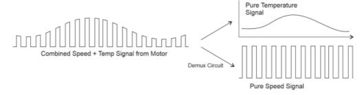
The Phaserunner V6 can also work with combined temperature and speed signals that are present on the temperature input pin. If there are no speed pulses present on the Wheel Speed signal, and the temperature signal periodically drops to 0V, then the Phaserunner V6 will treat those 0V pulses as speed signals to track wheel rotation.
