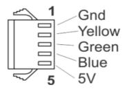
• The 3 Hall signals and 5V Hall power are provided through the 5 pin female JST-SM connector. This is a user crimpable plug.
