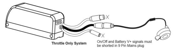
Finally, the Phaserunner V6 can be run with only a throttle on the Mains plug, or a PAS / Torque sensor plugged into the 6 pin PAS plug. In these arrangements, it is essential to wire up the on/off power switch on either the WP8 plug or the Mains connector for the controller to turn on, as outlined in Section 6.1.
