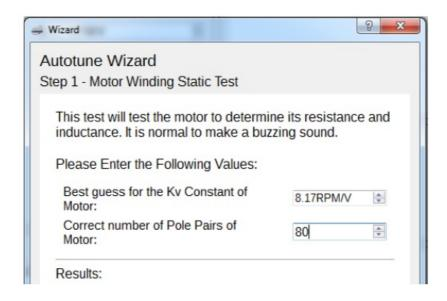
The start of the Autotune process asks for your best guess of the motor's kV in rpm/V, as well as the number of pole pairs in the motor. The firmware uses these initial parameters for determining the test current frequency.
