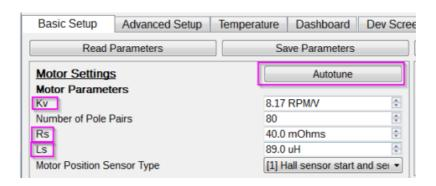
The Autotune routine can automatically detect motor parameters like the motor speed constant (kV), resistance of one motor phase to neutral (Rs), and the inductance of motor phase to neutral (Ls).
