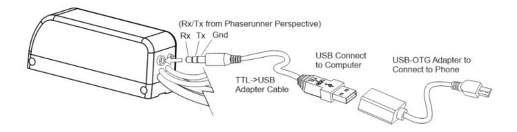
A TRRS jack embedded in the controller can be used for connecting to a computer, Android smart phone, or potential Bluetooth dongle (future product).
