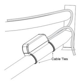
The Phaserunner is designed to be narrow in width and has a channel down the back of the heatsink so that it can be strapped to your bicycle tubing with a pair of cable ties. When mounted externally like this, the controller is exposed to abundant air flow for cooling.
