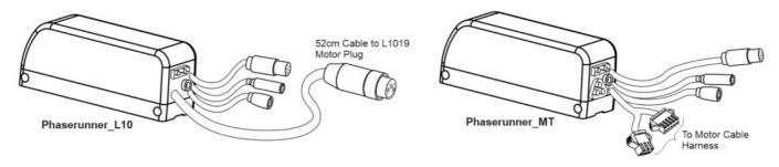
This manual covers two production models: the Phaserunner V6\_L10 and the Phaserunner V6\_MT. The L10 model is intended for motors already using the L1019 connector, while the MT model employs a cable harness between the controller and motor for accommodating various other connector standards.
