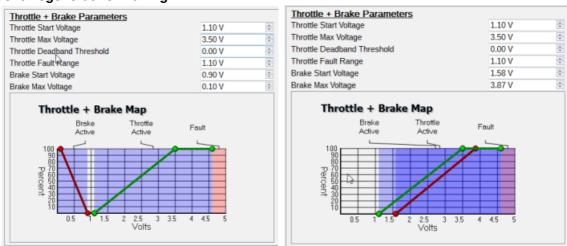
The Phaserunner V6 by default has both the throttle signal source and the regen brake signal source coming from the same line, Analog Input 2, which floats at 1V when disconnected. This allows for a single wire to control both power and braking. The signal can be shorted to ground via an ebrake lever to achieve maximum regen braking.
