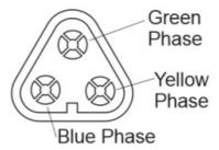
The MT60 connector supports 3 phase power in a single plug. These connectors can be readily soldered for making custom harnesses.
