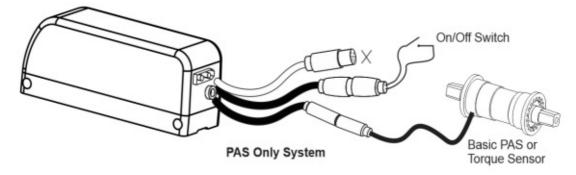
This minimal approach with a PAS sensor does not provide for any means to adjust the assist level outside of reprogramming the controller, and for that reason has limited usefulness. A display unit with up/down buttons is required in order to vary the amount of assist while riding.
