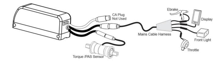
The Phaserunner V6 can be used with certain third party displays (from King Meter, Star-Union, Bafang etc.) that communicate using the KM5s and other supported digital protocols. This is achieved with a 9 pin Mains cable harness which splits out the 9 signals into separate plugs for throttle, display, ebrakes, and front light, along with an (optional) PAS or Torque sensor hooked up to the 6 pin PAS plug as well.
