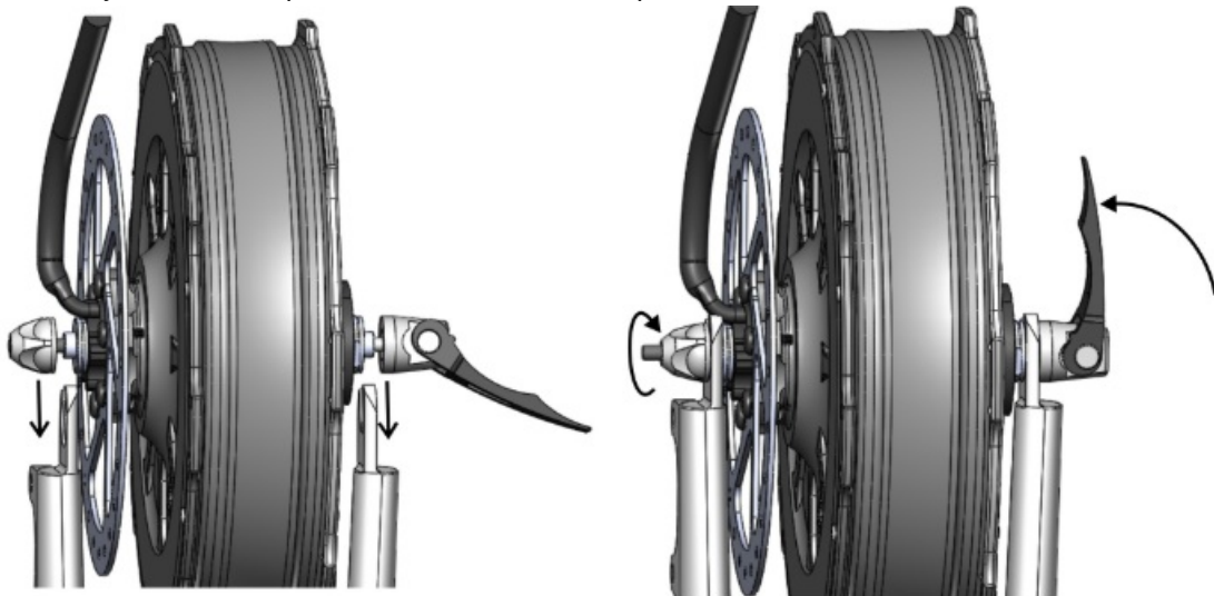
Figure 8: Install hub with torque arm behind fork blade. Ensure that cable exits down and out of dropout slot without getting pinched.
