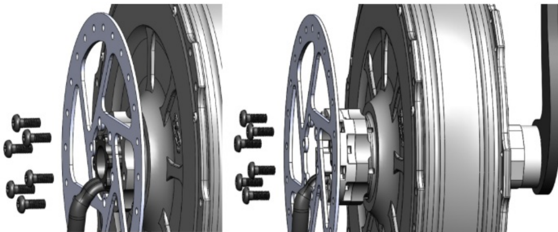
Figure 6: Mounting the Disc Rotor, Standard (left) and Fatbike (right). A narrow 1.5 mm spacer may be used under disc rotor for larger caliper clearance. See Section 8.2 Disc Caliper Clearance.
