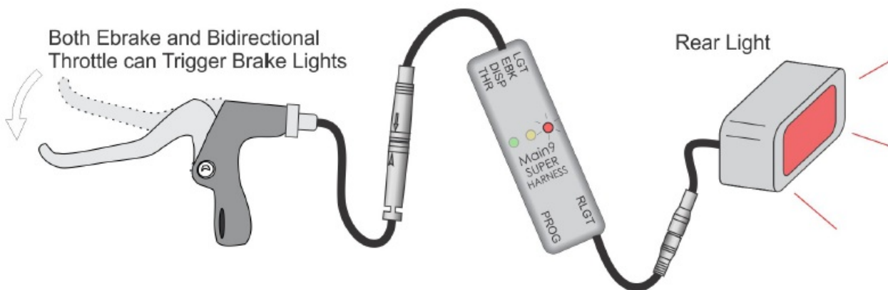
Figure 12: The rear light port can be used as a brake indicator in modes 3, 4, and 5.
