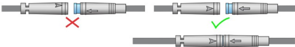
Figure 3: The alignment arrows can be subtle and hard to see. Jamming connector when missaligned can damage pins.
