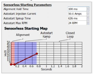
As initial values, set the "AutoStart Injection Current" to half your maximum phase current, an "AutoStart Max RPM" about 5-10% of the running motor rpm, and an "AutoStart Spin up Time" anywhere from 0.3 to 1.5 seconds, depending on how easily the motor can propel the bike up to speed. On bikes that you pedal to help get you underway, a short 0.2-0.3 second ramp will often work best,
