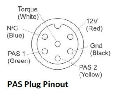
The V4 Baserunners include a 6 pin HiGo MiniB Z609 plug for direct connection of a PAS sensor or Torque Sensor, even without the use of a Cycle Analyst device.
