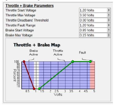
With the brake and throttle lines tied together into a single signal, the Baserunner can support variable regen either through bidirectional throttles or a V3 Cycle Analyst.
