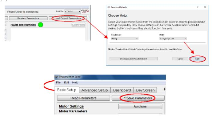
Install these new settings to the Baserunner via the "Save Parameters" button. Apply some throttle and your motor should run smoothly. If so, you can now skip over the "Motor Autotuned" section, and proceed to "Battery Limits." If your motor is not listed on the "Import Defaults" window, try choosing "Download Latest Defaults from Grin" and follow the prompts. If default settings for your motor are still not available, proceed to the "Motor Autotuned" section that follows.
