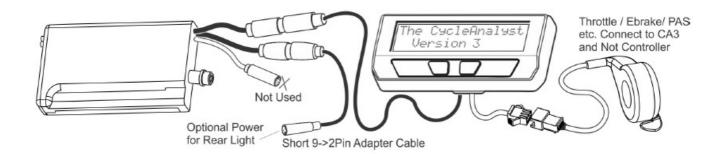
The CA3-WP device is plugged into the matching connector. All throttles, ebrakes, and PAS or Torque sensors are plugged in directly to the Cycle Analyst.
