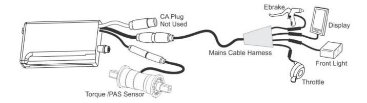
At present Grin only provides support for this hookup to OEM customers purchasing complete systems with 3rd party displays using the KM5s protocol, and does not offer support or the components for this at the retail level. In this wiring approach, the 8 pin CA-WP plug is not required, but it can be used as a convenient tap point to power a rear bike light as well.
