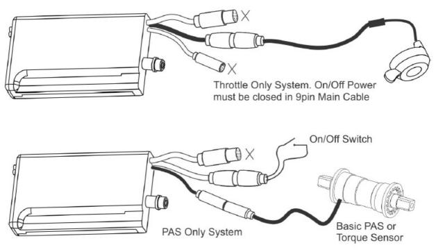
There will not be any ability to modulate the PAS power assist level or other system behavior in this minimal approach.
