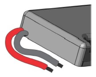
The short 5cm leads for the battery pack emerge on the back end of the controller. When supplied with a downtube battery these leads will be soldered to the mating cradle connectors, while they may be unterminated or fitted with Anderson Power poles when purchased alone.
