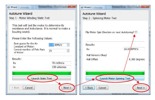
During the spinning test, the Baserunner will start the motor in sensor less mode. If the motor fails to spin and just starts and stutters a few times, adjust the sensor less starting parameters as described in section 5.5, "Tuning the Sensor less Self Start," until the motor is spinning steadily.
