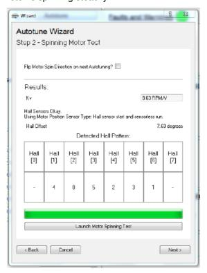
If the spinning test detects a valid hall sequence, the final screen will show the hall offset, and that the "Position Sensor Type" is "Hall sensor start and sensor less run."
