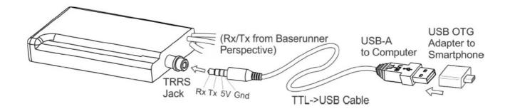
The communication standard uses a 0-5V level serial bus. Grin sells a 3m long TTL->USB adapter cable to connect the unit with the USB port of a standard computer. This is the same communication cable used with the Cycle Analyst and Satiator products. Third party USB->Serial cables, such as FTDI's part number TTL-232R-5V-AJ are also compatible. A USB-OTG adapter then is needed to connect to an Android smartphone via the phone's smaller Micro USB or USB-C port.
