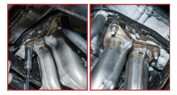
7. White supporting the header, carefully remove the last two nuts holding the factory header onto the heads. The factory header should now be able to come straight down and off of the vehicle.
