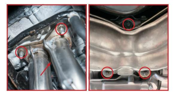
3. Locate the front side of the turbo, between it and the radiator, and remove the 10mm bolt that holds the heat shield.
