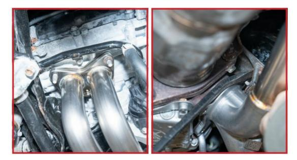
10. Because the supplied replacement turbo studs do not have Torx heads, use the best remaining OEM stud for the upper position and the new studs for the bottom two. Torque these studs to 11 ft/lbs. Ensure the upper stud passes through the heat shield.
