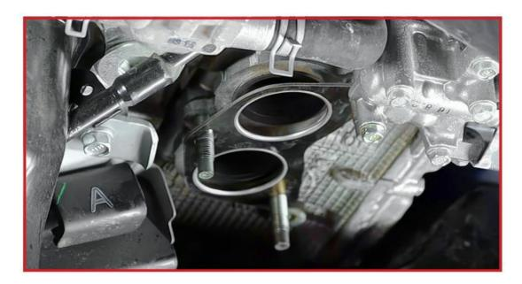
9. Take your Grimmspeed Header as well as the supplied turbo gasket and lift them up into place under the engine. Loosely install the included replacement nuts onto the studs in the heads, but do not fully tighten them yet. You may need to gently pry the turbo shield to get the header to seat in place on the turbo flange.
