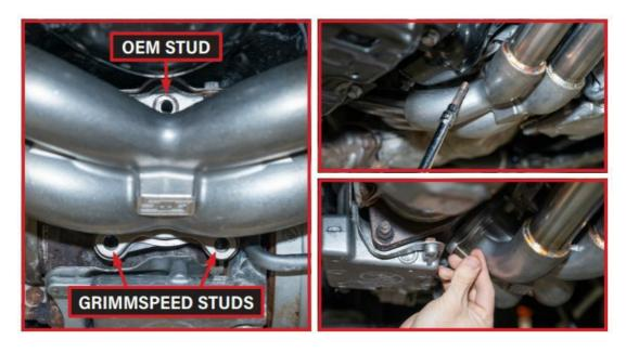
11. Once the turbo studs are installed, install the three included M10 nuts and torque them to 31 ft/lbs.
