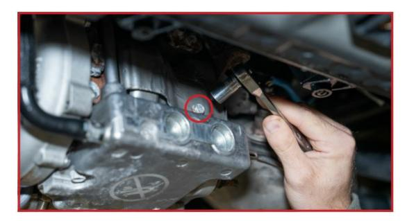
4. Use a deep 14mm socket to remove the three nuts holding the manifold to the turbo. Access the upper nut by maneuvering an extension between the oil pan and manifold.
