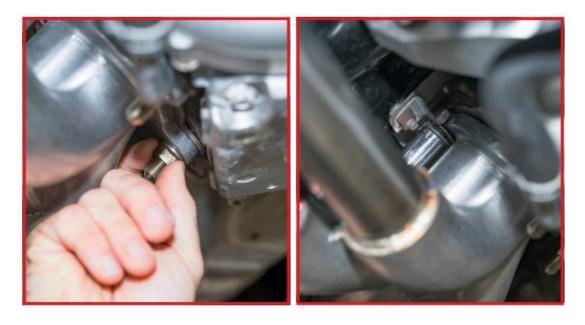
12. With the turbocharger secured to the new GrimmSpeed manifold, you can now fully torque down all six nuts attaching the header to the heads of the engine. These nuts will be torque to 47 ft/lbs following the sequence outlined below.
