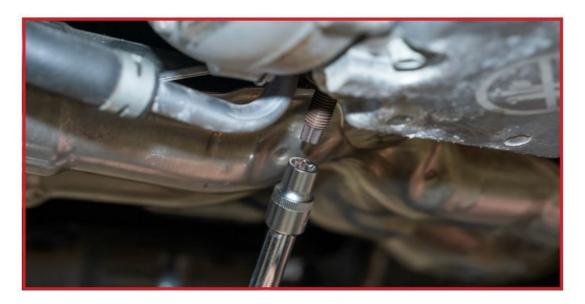
6. Remove the six 14mm nuts attaching the manifold to the heads. Leave one nut loosely threaded on each side to prevent the manifold from falling when removing the last nut. You will need to use an extension and reach in between the runners to get at the inner nut on each side.
