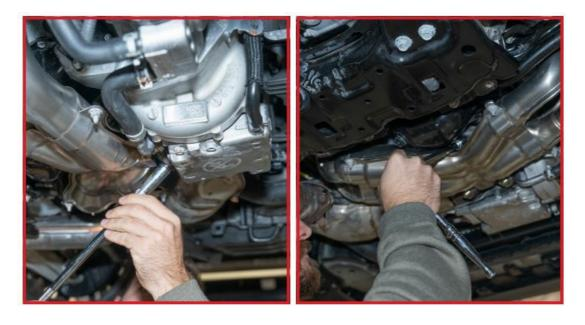
5. Carefully remove the three turbo studs with an E10 torx socket, taking care not to snap the studs. We highly recommended to use a ratchet instead of power tools to avoid snapping the studs. If you experience resistance, apply penetrating oil and consider heating the area around the studs. We recommend running an M10x1.25 tap through the threads in your turbo to ensure that there is no damage to the threads.
