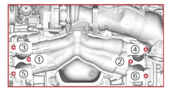
13. Start the vehicle and check for exhaust leaks, taking caution as the exhaust will heat up quickly. If there are no exhaust leaks, you can reinstall the skid plate and plastic under body cover and hit the road! We do recommend double checking the torque settings on the head nuts after a few heat cycles just to verify that everything is still tight.
