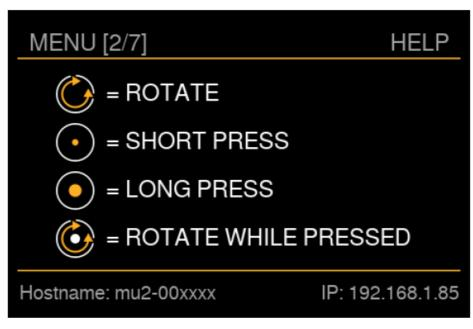
This menu shows the pictograms that are used in the MU2 for operating the main knob. At the bottom of the screen the current network information is shown. The indicated hostname depends on the serial number of your MU2.
