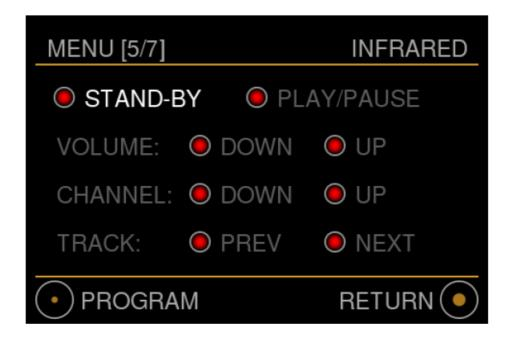
The dot will turn orange until the MU2 receives an infrared command. Press the desired button on your infrared remote to link this infrared command to the selected function.
