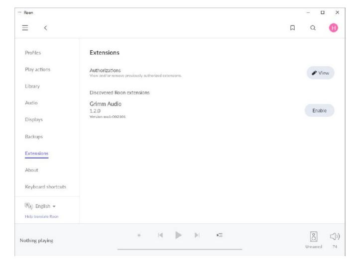
To activate the extension, go to the tab Extensions and press Enable for the Grimm Audio extension. You may press View to see the active extensions. Make sure there is only one activated Grimm Audio Extension. After this step your MU1 is ready for use.
