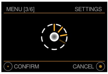
Turn the main knob clockwise to increase the brightness and anti-clockwise to decrease the brightness. Please note that the LED can not be turned off completely to facilitate showing whether the MU1 is in operation/standby or powered off.
