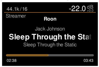
If an LS1 is connected, the MU1 will send volume control data to the DSP of the LS1 via its proprietary cat5 cable. If the volume control is activated for one or more digital outputs, the FPGA chip performs a volume attenuation at high precision for these output(s). See 'Settings menu [3/6]' for selecting volume control on the digital outputs.
