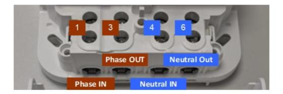
All terminals are clearly, unequivocally and indelibly indicated in the meter on its front face in proximity of the output terminals. They are marked from left to right (with the meter in operating position) showing the function of the connected wire as follows:
