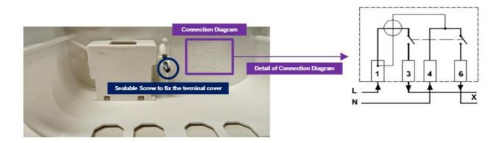
The input/output terminals support cables with a cross section between 4 and 50 mm2. The fixing screws of the cables must be tightened with a torque of 6 Nm.
