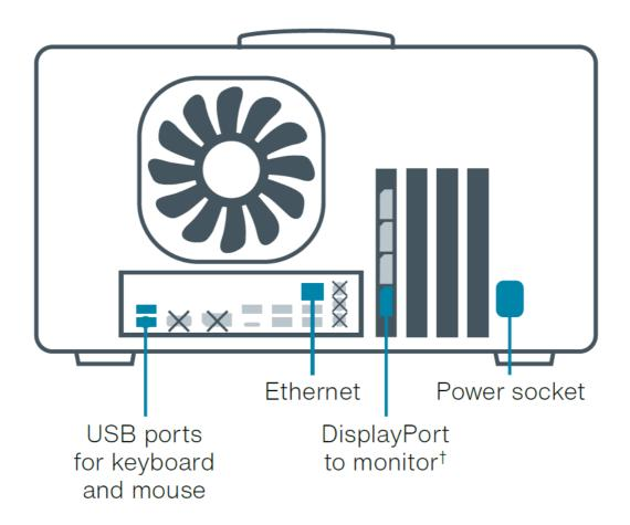
Only use the ports and connections coloured in blue for installation.
