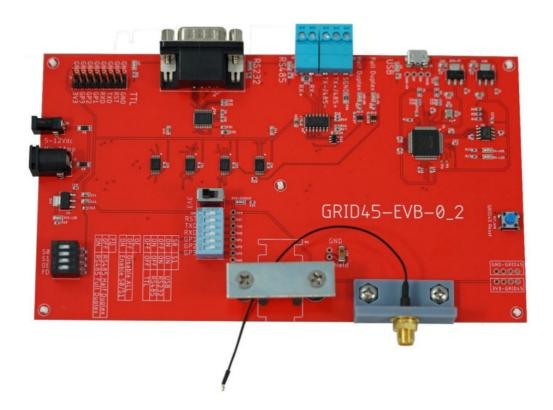
module. The evaluation board uses a multiplexor circuit to provide four optional, external serial connection options to the single serial interface on the GRID45 module. This allows OEMs to test the GRID45 in any one of the following modes:
