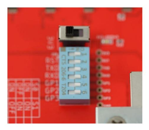
This switch controls the +3.3-volt power source to the GRID45 module to powered On or Off.
