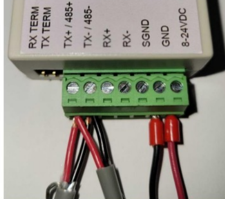
2-Wire Daisy-Chain, No SGND, No Termination
