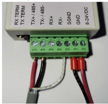
2-Wire, with SGND and Termination
