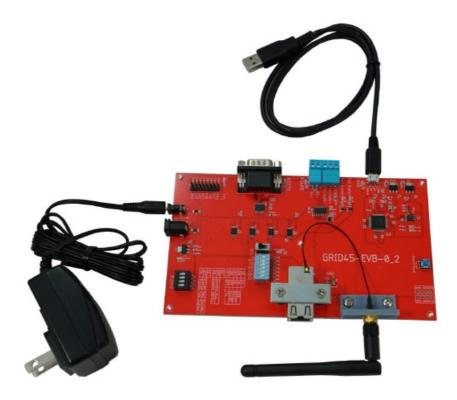
The GRID45 Evaluation Board provides a flexible test and qualification platform for all variations of the GRID45 module. The evaluation board uses a multiplexor circuit to provide four optional, external serial connection options
