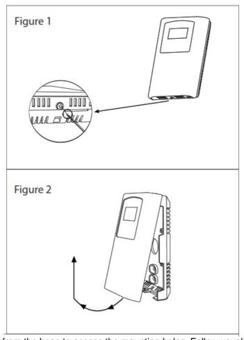
The PCB must be removed from the base to access the mounting holes. Follow usual anti-static procedures when handling the PCB and be careful not to touch the sensors. The PCB is removed by pressing the enclosure base to unsnap the latch near the bottom edge, then the PCB can be lifted out of the base as shown in Figure 3.
