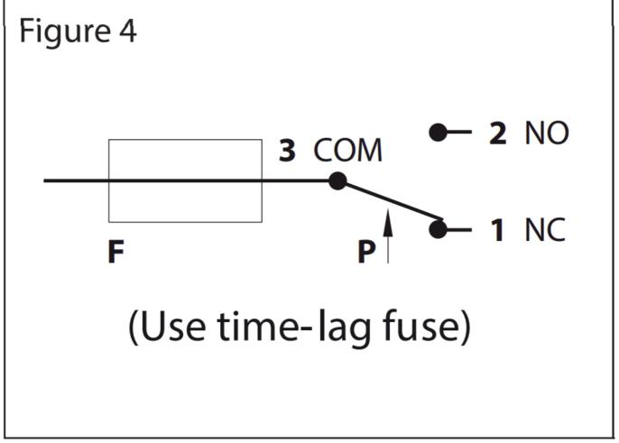
Max. 1.0 A / 250 VAC 50-60 Hz, at ohmic consumers. Max. 0.4 A / 250 VAC 50-60 Hz, at inductive consumers. Max. 0.1 A / 24 VDC 50-60 Hz, at the low-voltage version.
