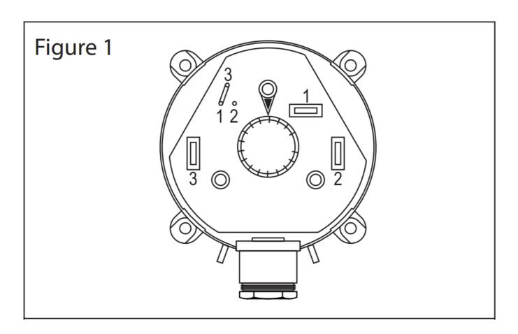
The connections are intended for 6.3mm crimp-type-sockets. Assemble flex- and solid wires accordingly. See **Figure 2.**
