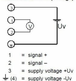
The type of current or voltage output is set by works and cannot be changed.
