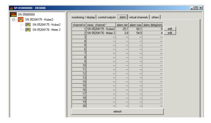
Here you can examine and redefine the adjusted alarm limits for each measurement channel. By pushing the "edit" button next to the respective measurement channel you reached a second dialogue window.
