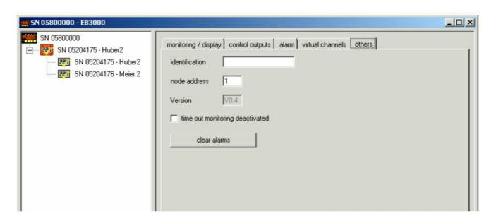
Here you have the ability to determine a device identifier and a node address. Furthermore, you can deactivate timeout monitoring and clear alarms. Additionally, you can see the version number of the EB3000.
