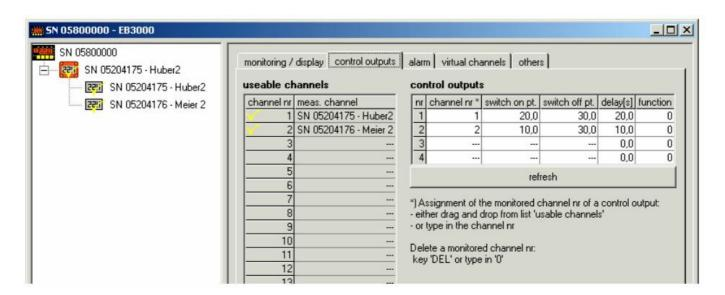
Here is once again a listing of the measurement channels with allocation to the control outputs. A modification or reselection of the channels results via "drag and drop" or through manually input of the respective channel number.
