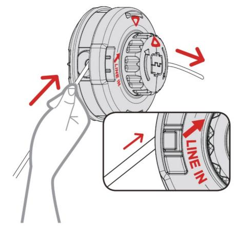
4. Pull the cutting line through until there is an equal quantity of cutting line on each side.
