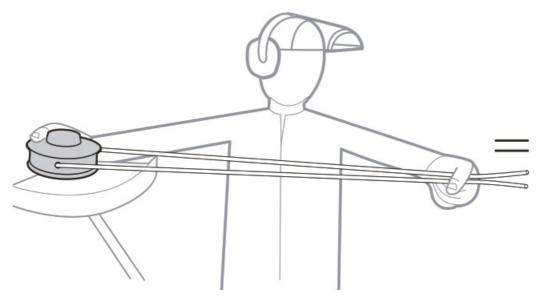
5. Turn the spool cap clock-wise to wind the cutting line into the trimmer head. Keep approximately 5 in of cutting line above out of each side of the trimmer head.
