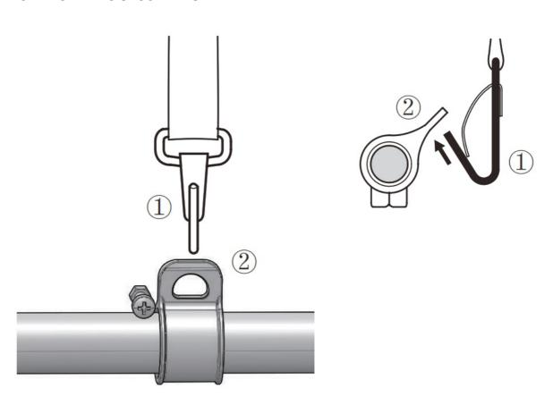
1. Attach the carabiner to the carrying ring on the drive tube.
