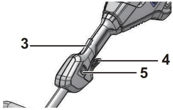
2. Push the speed switch (5) to the desired operating speed. Push the speed switch to position 1 for low speed or position 2 for high speed.
