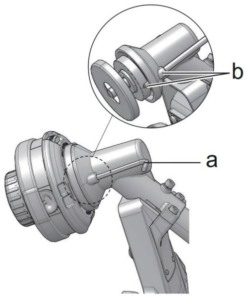
2. Turn the trimmer head clockwise to loosen it. Do not remove the spacer from the shaft.
