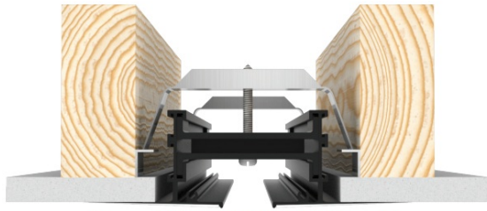
Figure 17 (Step 5A): Install Drywall – Exposed Face/Flange Border (A)
