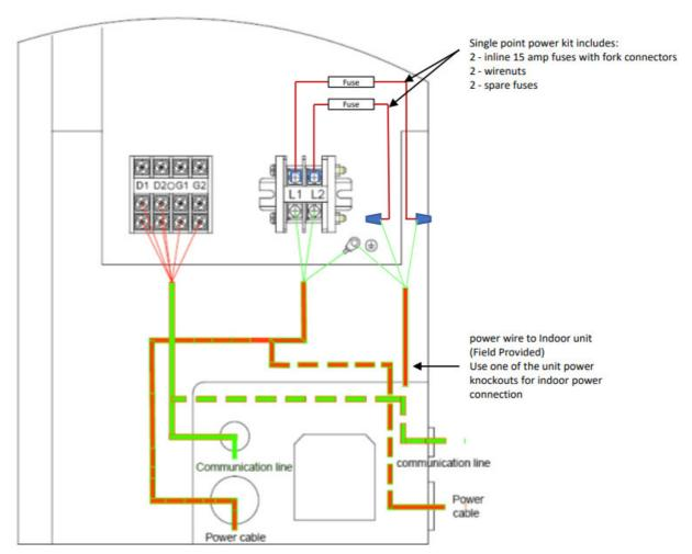
Control wire and power wire should be run in separately to avoid communication interference Outdoor unit MCA and MOCP values do not need to be adjusted when using this kit
