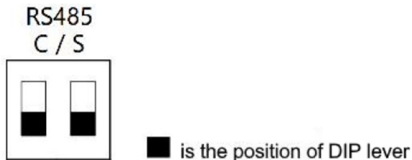
Figure 3.10 Primary Station Setting Diagram
