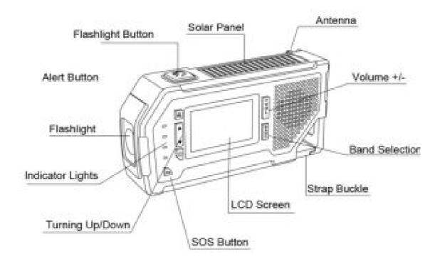
► Indicator Lights (From top to bottom: Charging indicator, Signal indicator, Power indicator, Alert indicator)
