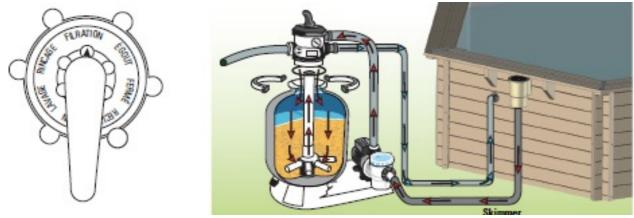
2. **WASHING POSITION (OR BACKWASH):** Sand washing position. Allow the water to circulate in reverse direction in the filter. The water enters through the lower part of the filter elevates the filtering mass and therefore collects all its impurities and because they are lighter than sand, they area evacuated through the upper part of the filter towards the drain. This operation should last between 2 and 3 minutes.
