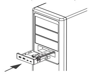
2. Fix the front panel with the supplied screws.
