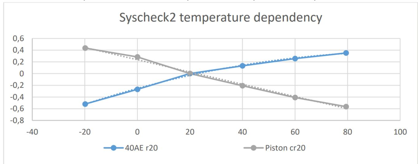
40AE r20: is the Syscheck2 measurement with the load of 40AE Piston cr20: is the measurement of the 40AE sourced by the pistonphone.
