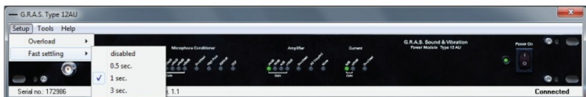
Fig. 7. The 12AU's fast settling modes
