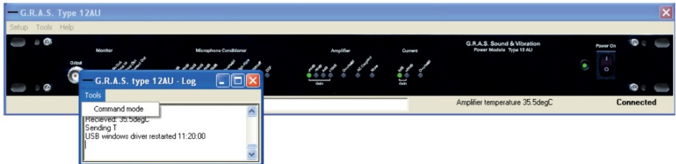
Fig. 19. The G.R.A.S Type 12AU log window is accessed from the Tools menu. Here you can enter commands and view responses. When command mode is used, the graphical user interface disappears from the screen.
