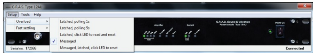
Fig. 6. The 12AU's overload handling modes
