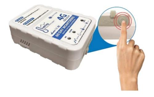
2. Normal Operation – After turning the device on, the device will send data according to the pre-set 15-minute interval, and "OK LED" will flash a green light every 10 seconds or press the "Button" key "OK LED" to flash the green light once and "wake up" the device.
