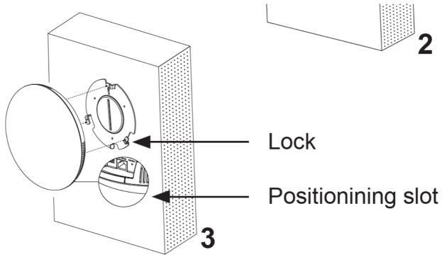
4. Rotate the device clockwise untill it is locked on the right postion.
