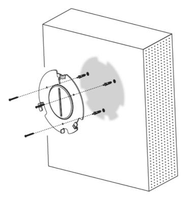
3. Align the position line on device's back cover with the positioning slot.
