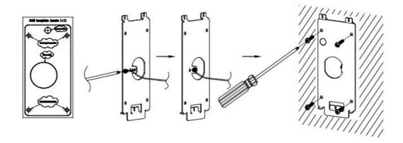
**Step 2:**Pull Cat5e or Cat6 cable (not provided) through the rubber gasket selecting the correct size and the back cover panel piece, please refer to GDS3702 WIRING TABLE at the end of QIG for Pin connections.
