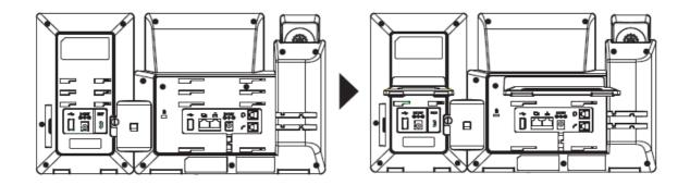
**Note:** In case two or more GBX20 extension modules are connected to the GRP2615/GRP2624/GXV3350, the second GBX20 needs to be powered on by a 12V/1A PSU.
