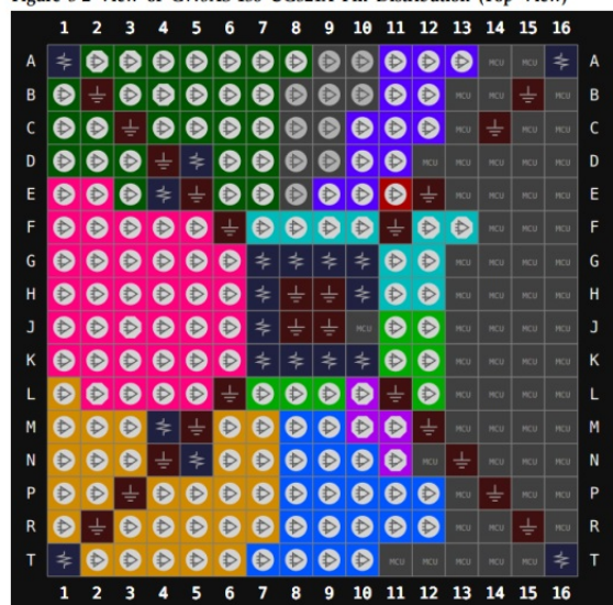
Figure 3-2 View of GW5AS-138 UG324A Pin Distribution (Top View)
