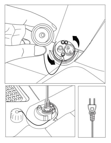
Unplug the charger and screw the plastic cap onto the device ensuring a firm fit. Now you're ready! **WARNING:** Do not operate the device out of the water as it may damage some components.
