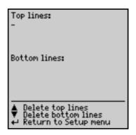
From the keyboard, you can enter optional texts which – before and/or after the test result – are to be automatically included in the report printout.
