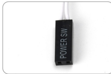
Power switch port
