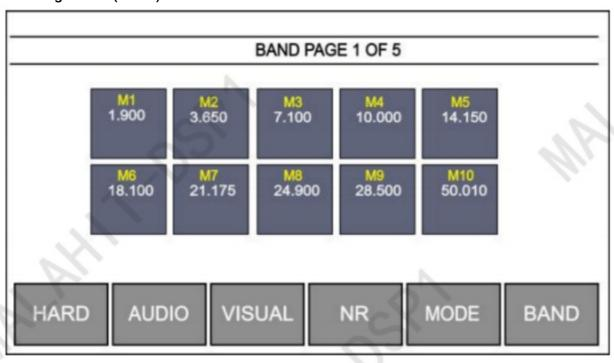
The BAND menu is used to save and read the radio's settings. Click on the BAND icon to open the menu and click on the BAND icon again or clte:k on the EXIT icon to exit the menu. The tabs are laid out on a page-by-page basis and are turned by turning the Frequency knob.
