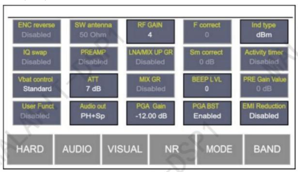
This HARO menu allows you to configure various hardware features such as radio frequency gain, preamplifiers, attenuator5i, and more. Touch a menu item to select n:. If an item has more than two different values, rotate the FREQUENCY knob to toggle between these values. To exit the menu, touch the HARD button again. The menu includes the following items:
